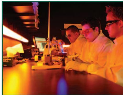
*This team is testing resin curing lights to determine their ability to cure a variety of resin-based composites. CR has demonstrated that proper light alignment can greatly affect resin curing light performance.*
